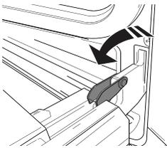
**2.** Close the door as much as you can. Take a firm hold of the door with both hands – do not hold it by the handle. Simply remove the door by continuing to close it while pulling it upwards (a) at the same time until it is released from its seating (b).
